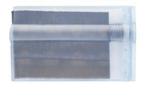
GRAPHIC BLADE NO. 8605 from MARTOR is a high-quality blade made of steel with TiN-coating. It is very sharp and has one usable cutting edge. The blade is 32.5 mm long, 5.7 mm wide and 0.50 mm thick.
