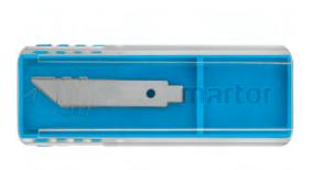
GRAPHIC BLADE NO. 680 from MARTOR is a high-quality blade made of steel. It is very sharp and has one usable cutting edge. The blade is 37.5 mm long, 6.1 mm wide and 0.50 mm thick.
