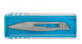
GRAPHIC BLADE NO. 34 from MARTOR is a high-quality blade made of steel. It is very sharp and has one usable cutting edge. The blade is 36.5 mm long, 5.7 mm wide and 0.50 mm thick.
