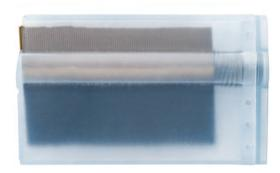
GRAPHIC BLADE NO. 8606 from MARTOR is a high-quality blade made of steel with TiN-coating. It is very sharp and has one usable cutting edge. Rounded tips increase user safety. The blade is 31.1 mm long, 5.7 mm wide and 0.50 mm thick.
