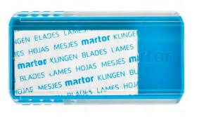
INDUSTRIAL BLADE NO. 37010 from MARTOR is a high-quality blade made of steel. It is very sharp and has four cutting edges that can be used one after the other for an extra long service life. The blade is 43 mm long, 22 mm wide and 0.10 mm thick.
