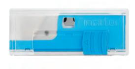
HOOKED BLADE NO. 98 from MARTOR is a high-quality blade made of steel. It is very sharp and has two cutting edges that can be used one after the other for a long service life. The blade is 54.8 mm long, 19 mm wide and 0.63 mm thick.
