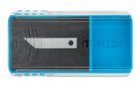
GRAPHIC BLADE NO. 834 from MARTOR is a high-quality blade made of steel with TiN-coating. It is very sharp and has one usable cutting edge. The blade is 36.5 mm long, 5.7 mm wide and 0.50 mm thick.
