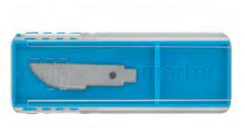
360° SWIVEL BLADE NO. 756 from MARTOR is a high-quality blade made of steel. It is very sharp and has two cutting edges for a long service life. The blade is 17.1 mm long, 19 mm wide and 0.50 mm thick.
