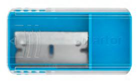
INDUSTRIAL BLADE NO. 60092 from MARTOR is a high-quality blade made of steel. It is very sharp and has four cutting edges that can be used one after the other for an extra long service life. Rounded tips increase user safety. The blade is 26 mm long, 18.5 mm wide and 0.40 mm thick.
