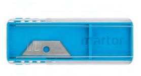
TRAPEZOID BLADE NO. 852 from MARTOR is a high-quality blade made of stainless steel with TiN-coating. It is very sharp and has two cutting edges that can be used one after the other for a long service life. The blade is 53 mm long, 19 mm wide and 0.63 mm thick. The oil used for the blade is food safe.
