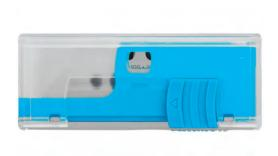
TRAPEZOID BLADE NO. 5232 from MARTOR is a high-quality blade made of steel. It is very sharp and has two cutting edges that can be used one after the other for a long service life. The wide ground edge makes cutting easier. The blade is 53 mm long, 19 mm wide and 0.63 mm thick.
